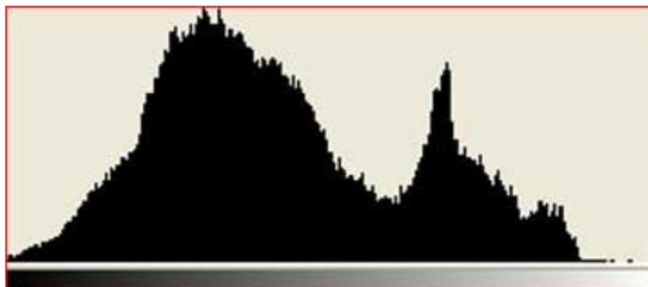
This histogram shows an almost perfect distribution of tones – from deep shadows on the left to just short of bright highlights on the right. This fits comfortably within the approximately 5 stop dynamic range capability of most digital imaging chips.
