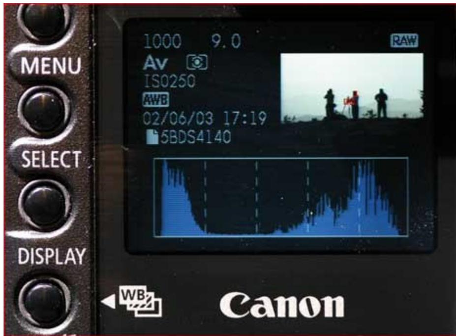
This view of the rear LCD on a Canon 1Ds shows a histogram for a particular shot and also the dotted vertical lines that Canon has engraved on the display separating the 5 stops of dynamic range that are available. As you can see this image has most of its content either in the shadows, or the highlights, with little in the mid-range.
