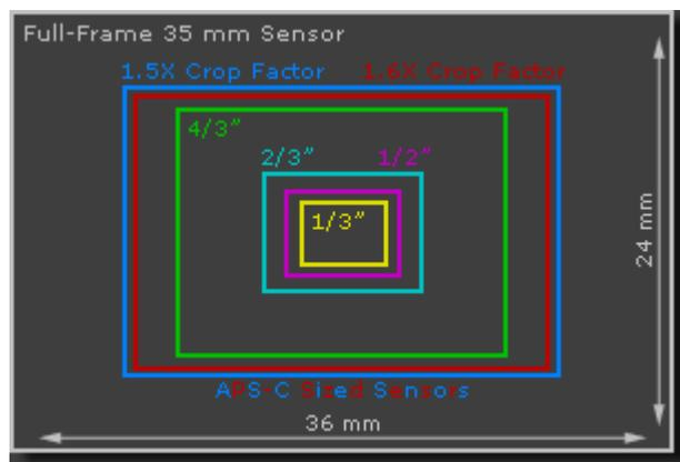
Canon's 1Ds/5D and Nikon D3 series are the most common full frame sensors, along with a couple of Sony cameras. Pentax and Olympus do not (2011) make them. Canon cameras such as the Rebel/60D/7D all have a 1.6X crop factor, whereas mainstream Nikon SLR cameras have a 1.5X crop factor. The above chart excludes the 1.3X crop factor, which is used in Canon's 1D series cameras.
