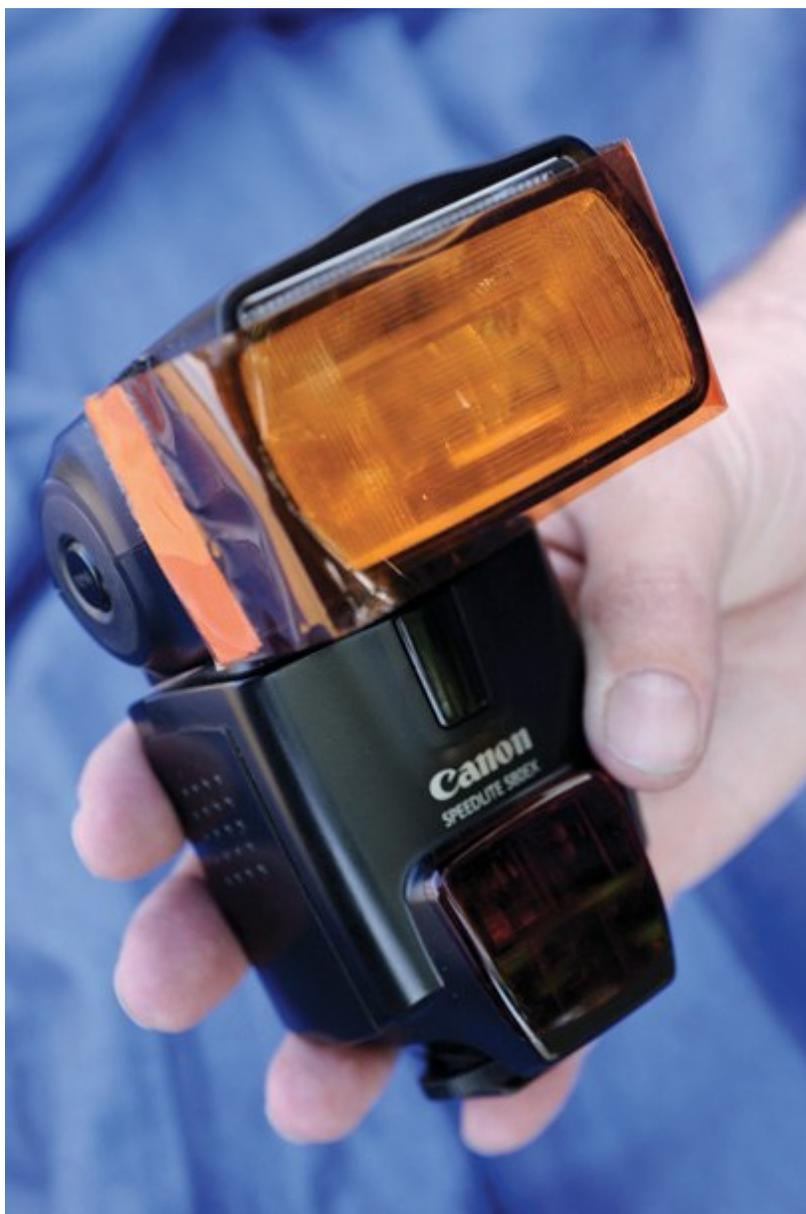
Use light balancing gel filters on flashguns to balance the light
