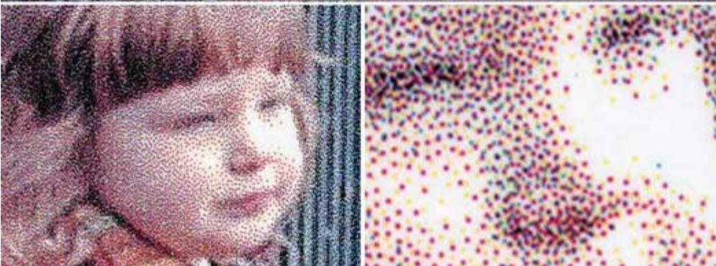
*This medium close-up (bottom left) of a typical inkjet print reveals the dot-dithering that makes up the printed detail that represents the image on the paper. Magnified further (bottom right) and you can see the individual dots of cyan, magenta and yellow ink formed as droplets of ink fired from the print head hit the surface of the paper.*
